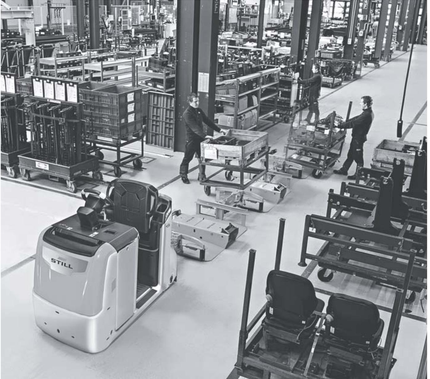
Maximum flexibility with B-Frames in confined working areas due to two-way loading and unloading options
